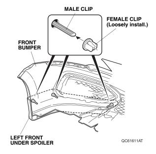
15. Remove two adhesive backings in the order shown. Press the left front under spoiler firmly against the front bumper with the palms of your hands to adhere the left front under spoiler.
